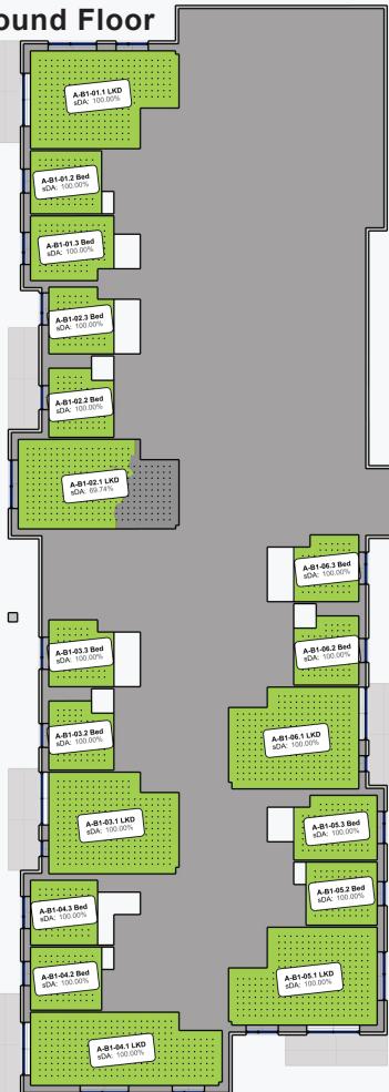
Figure 41: Block B1 - Floor plans indicating Daylight Provision to BS EN17037:2021+A1 Table NA.1
