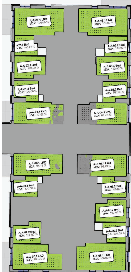
Figure 43: Block A1 - Floor plans indicating Daylight Provision to BS EN17037:2021+A1 Table NA.1
