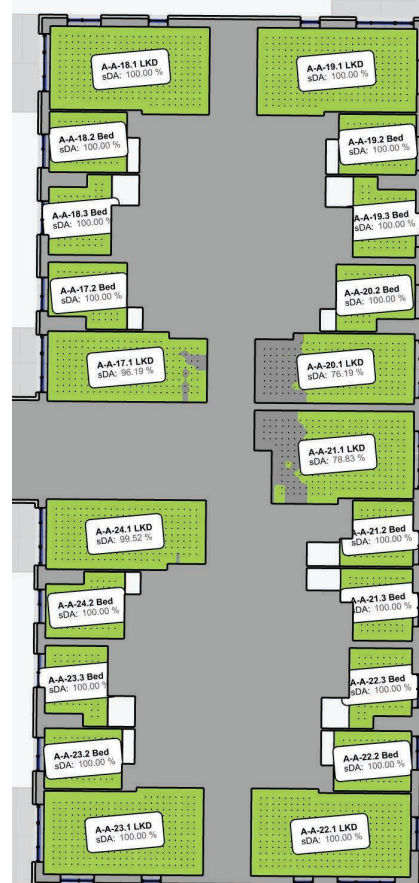
Figure 43: Block A1 - Floor plans indicating Daylight Provision to BS EN17037:2021+A1 Table NA.1
