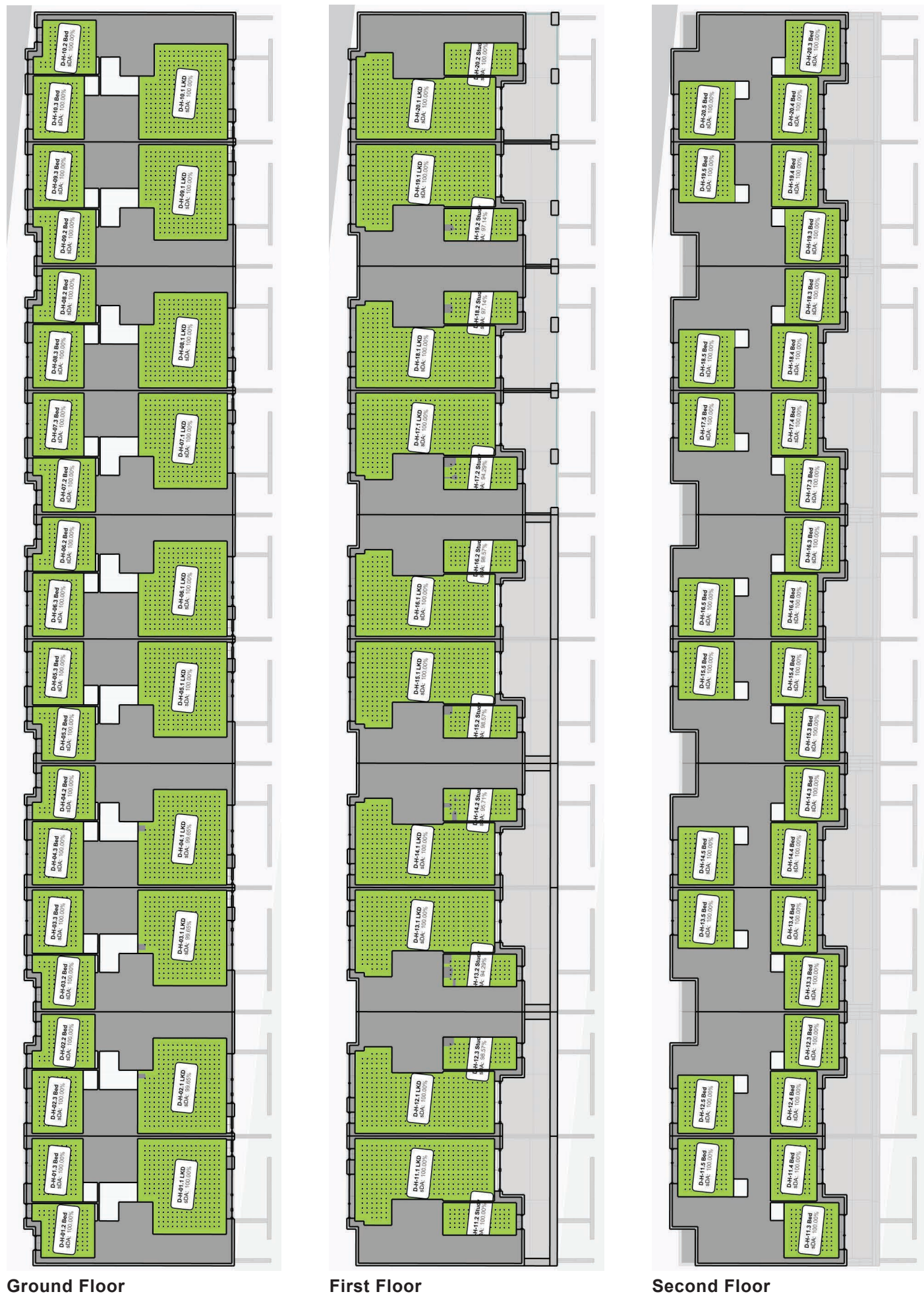
Figure 54: Duplex H1 - Floor plans indicating Daylight Provision to BS EN17037:2021+A1 Table NA.1
